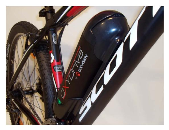
The battery holding unit should be fitted normally in the place of the water bottle cage. Most of the bicycles already have ready made frame decals where the water battery holding unit can be fitted.
