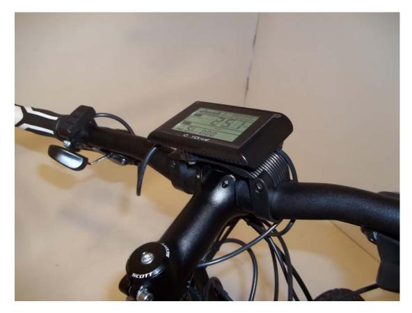
Fitting the throttle and the power setting buttons will depend on the type of the bike and this has to be tried by each user. Both throttle and the power buttons can be located on either left or right hand side of the handlebars.
