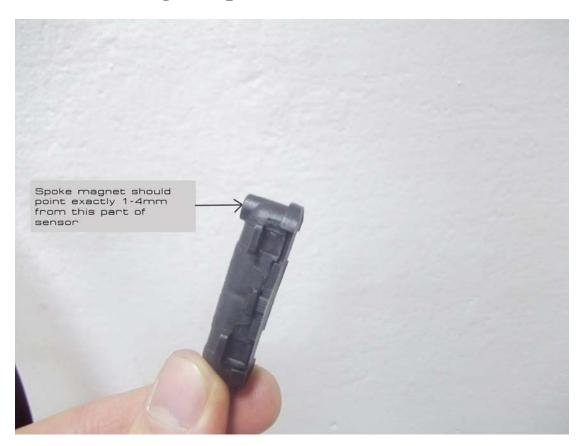
With the use of cable ties supplied with the kit attach the speed sensor to one of the forks legs. The spoke magnet should be installed on one of the spokes with the help of screwdriver. The magnet should point exactly at the point indicated by arrow at the above picture. The distance of the magnet from the sensor should be approx 1 to 4 mm.
