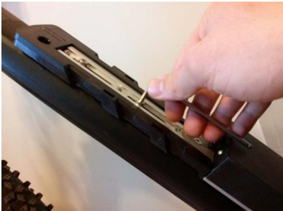
The battery holding unit should be fitted normally in the place of the water bottle cage. Most of the bicycles already have ready made frame mounts where the water battery holding unit can be attached to.
