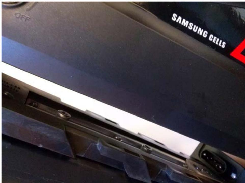
The battery should be slotted on the holder's rail and then drop down to connect with controller connector. Then battery should be locked with the key.
