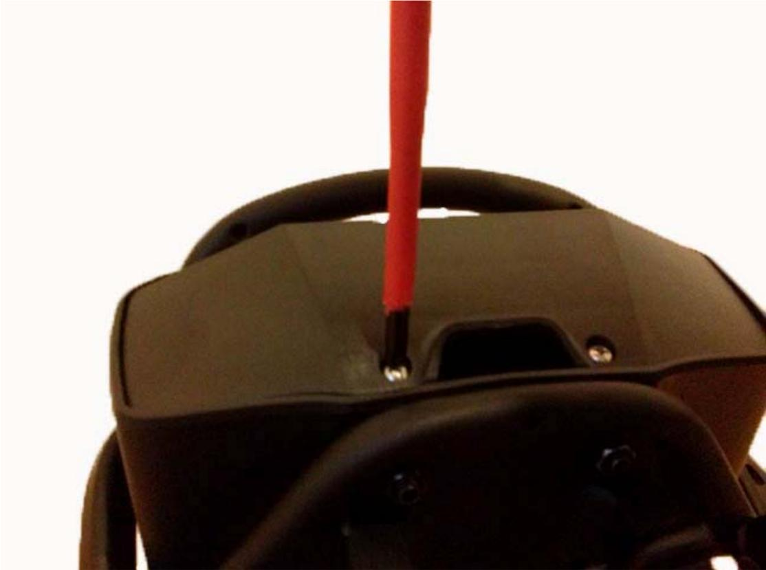
Open the lid from the controller compartment by using the screw driver
