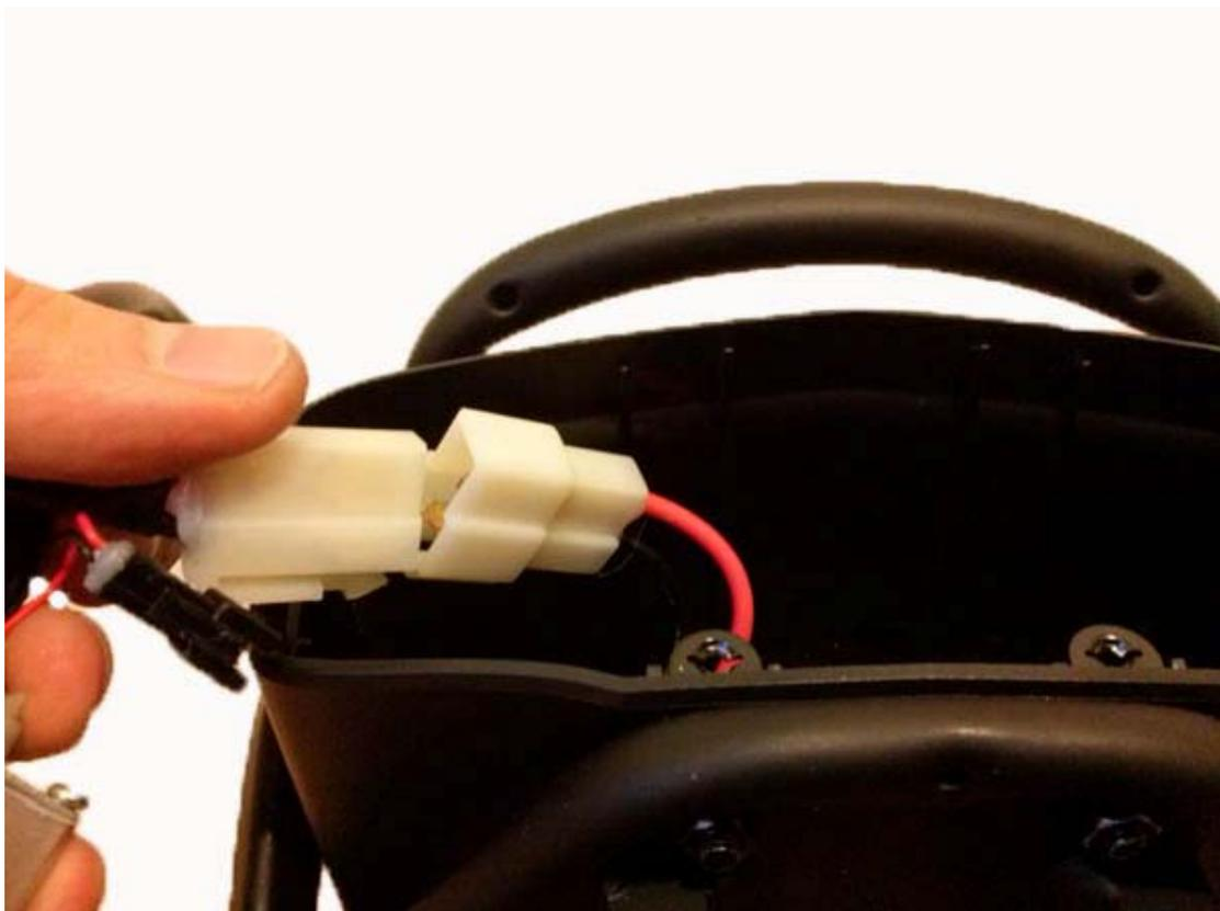
Connect the controller power connector with the battery connector. Connect other wires and slot in the controller in the controller box. Close the lid and fit the locking screws back again by using screwdriver.
